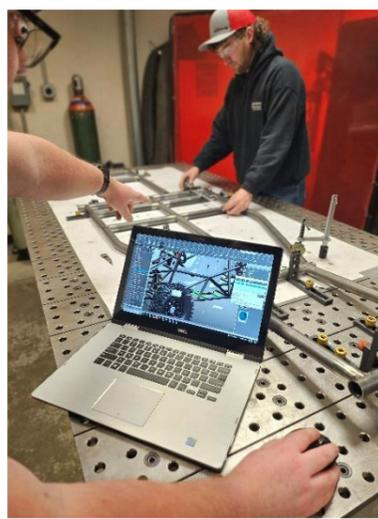
**SAE Baja Team** Fabrication has begun for the 2023-2024 vehicle. Over the past few weeks, the team has been working meticulously to cut, cope, and bend all tubular members for both the space frame chassis and front suspension members. March 25<sup>th</sup> is the target date for a completed vehicle. The team gives a big thanks to sponsors Wright Steel, NIX Companies, EBN, and Schmitt Metalworks.
