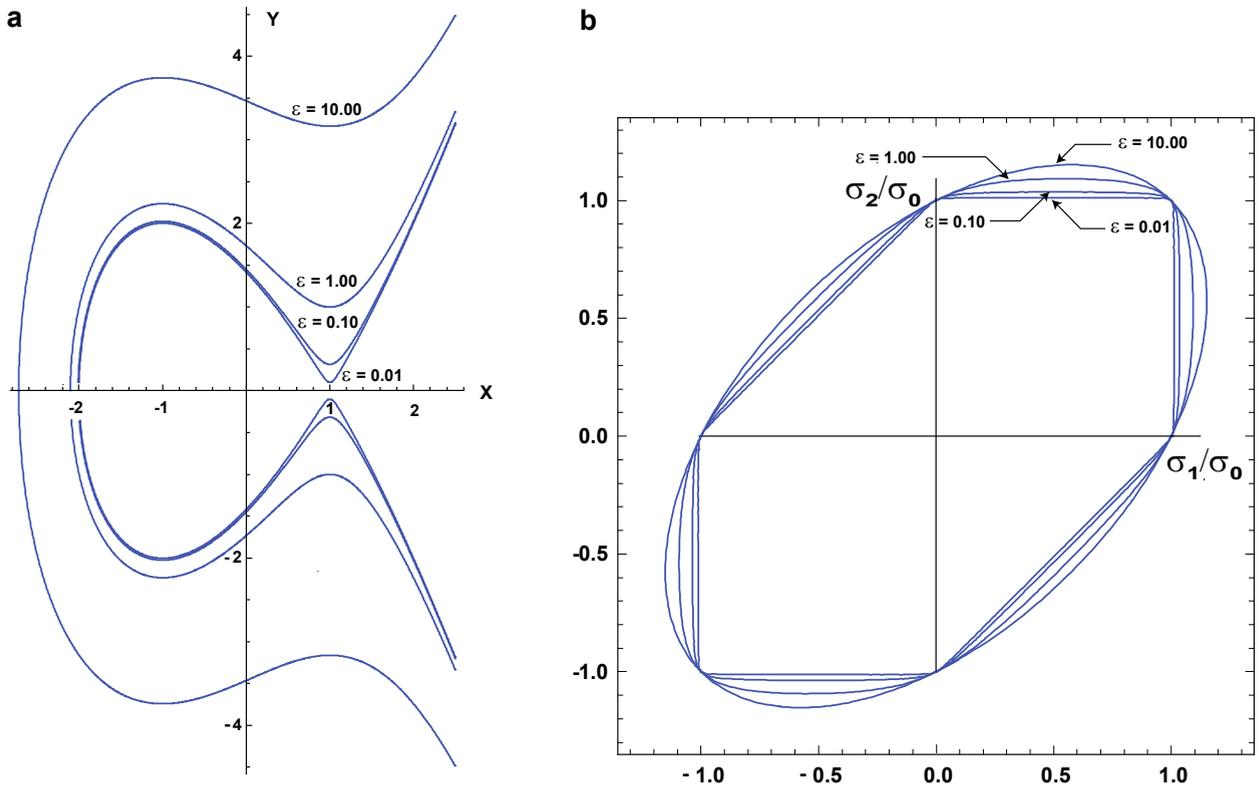
Fig. 3. (a) Elliptic curves of generalized Tresca yield condition; (b) generalized Tresca yield condition in normalized principal stress plane.
