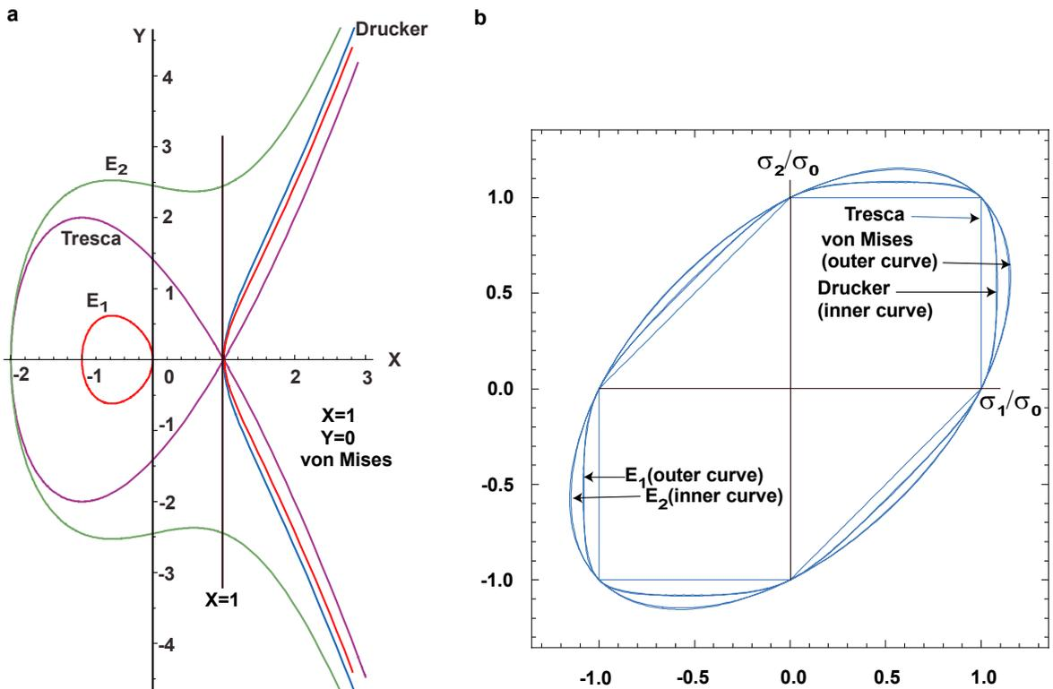
Fig. 1. (a) various yield conditions in the  $XY$  plane; (b) yield conditions in the normalized principal stress plane.
