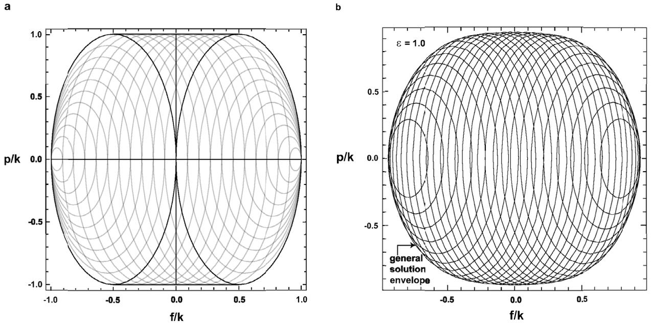
Fig. 2. (a) phase plane of solution of Tresca yield condition; (b) typical phase plane of solution of generalized Tresca yield condition.
