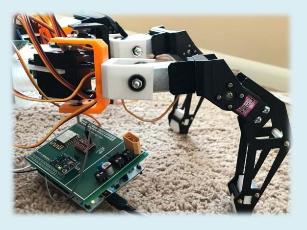
PCB circuit along with Maestro servo controller board used to drive the logic and to control all 18 servos.
