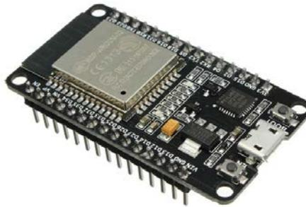
**Figure 5.** ESP32 development board
