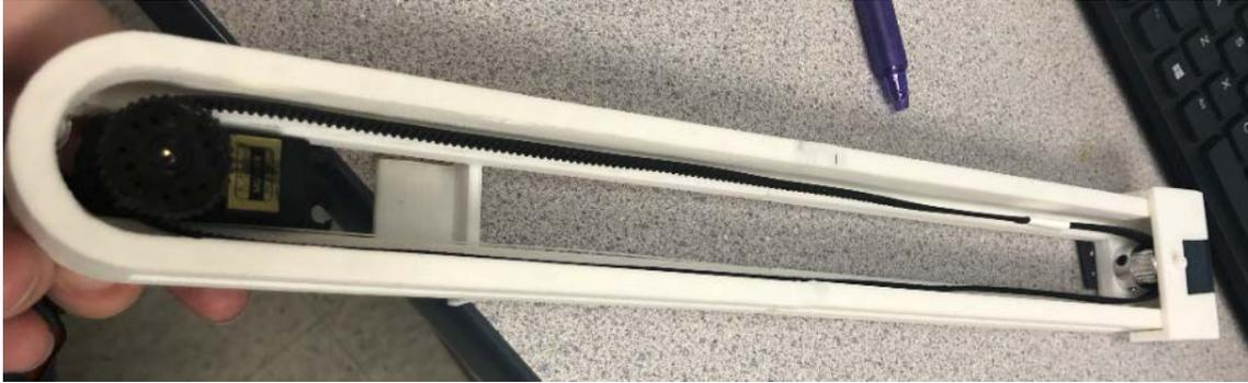
*Figure 9: Printed version of the vertical lifting pieces fitted together*
