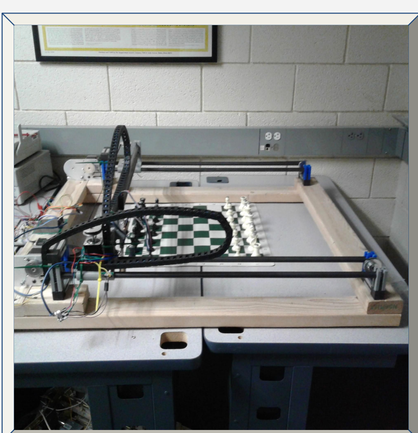
The robot can be placed over a chess set and is calibrated to the location of the board.
